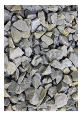
FIELD OF APPLICATION \_ Concrete and asphalt aggregate, cushioning filling of underground floor pipes
